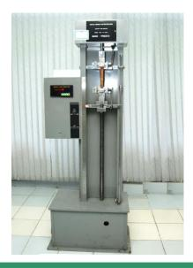
Test is carried out on vulcanized rubber sheet to determine the Tensile Strength and the % Elongation.
