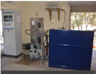
Computerized menu driven facility for measuring the water capacity of cylinder and conducting the hydrostatic test and burst test to determine the burst pressure and volumetric expansion of cylinder. Also has the facility for real time monitoring of the pressure and weight increase with time.
