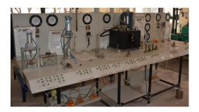
Automated Test Bench for SC Valve and Domestic Pressure Regulator
